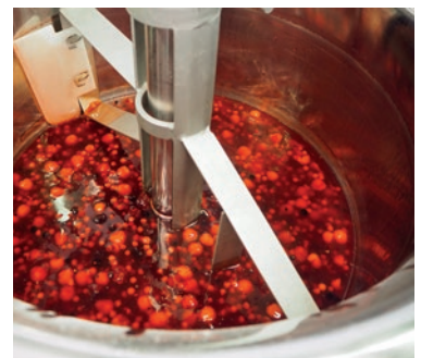
Strong, maintenance-free, auto-reverse mixer for all mixing, also whipping. Also available as a heavy-duty version for extra heavy loads.
