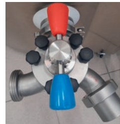
Three way arc valve
